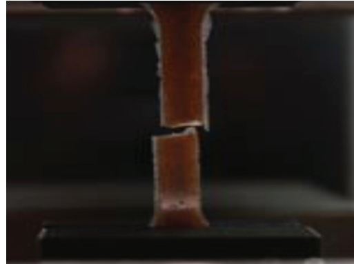
Fig.2: Specimen after tensile test
